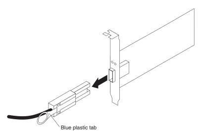
Figure 17. Removing a mini-SAS cable
